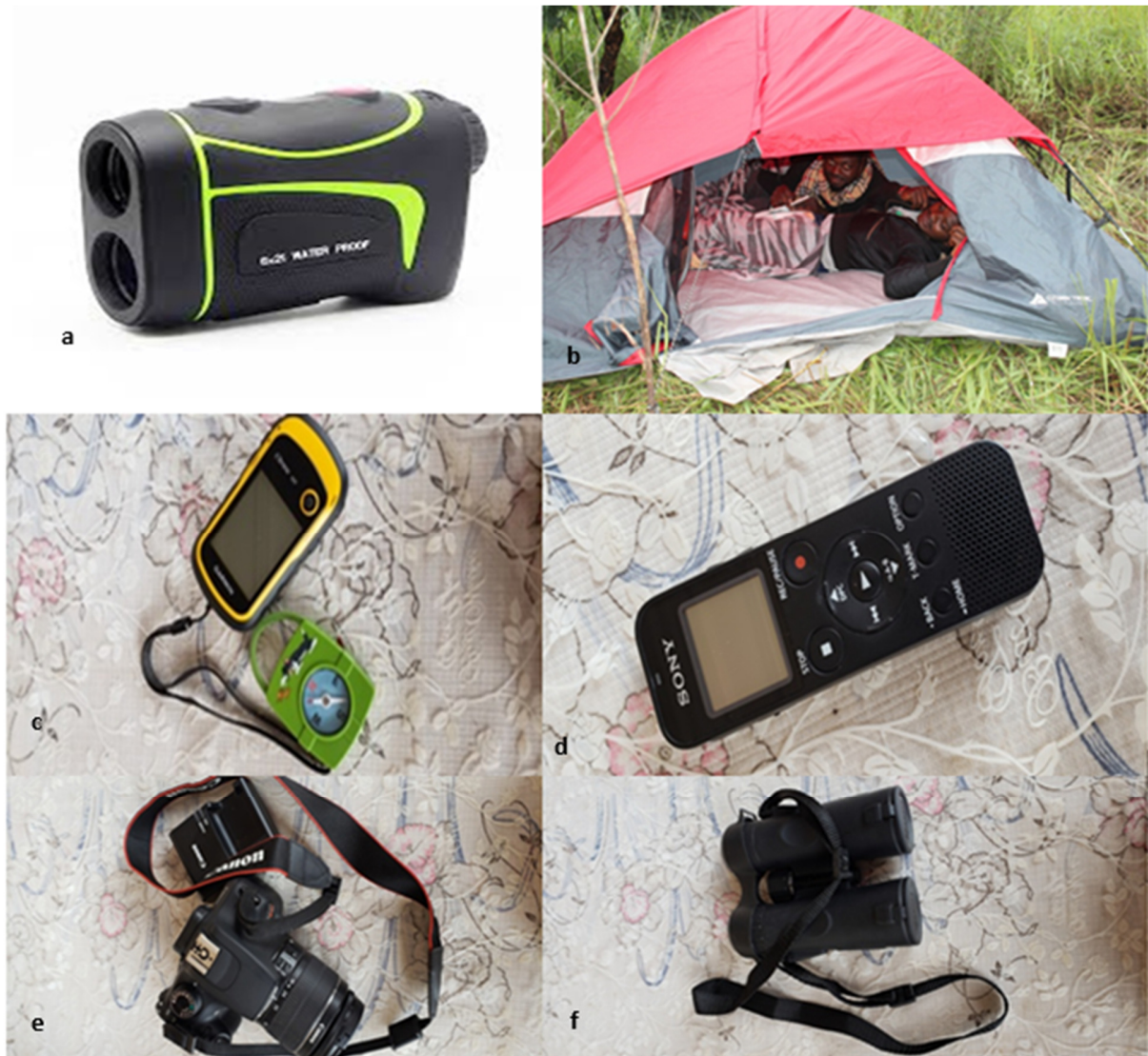
Figure 2 a-f. Materials used for field data collection. a. pair of rangefinders used for identification of species at varied distances. b. Refurbished tent used for lodging by the project team during field data collection. c. Garmin eTrex GPS and compass (for geographical coordinates and determining the North, respectively). d. MP3 Sound recorder (for recording bird sounds) during field activity. e. Canon digital camera for photos of birds and other features. f. Pair of binoculars for observing and identifying birds and other features at distances.
